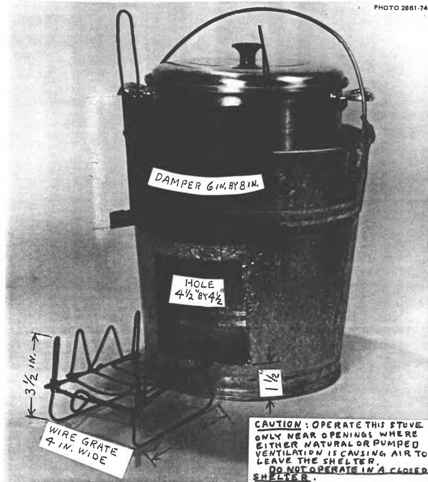
Fig. 4.37a. Expedient Bucket-Stove, made of a bucket, coat-hanger wire, about 2 ft of finer wire, and metal from an ordinary juice can. This is the most efficient expedient stove tested to date.
